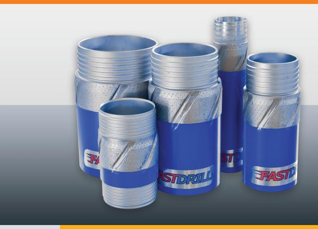
Reaming shells are designed to be placed behind the drill bit and the core barrel to ream the hole. A reaming shell has to be replaced when its diameter becomes less than that of the new bit to be introduced in the hole. This is intended to avoid new bits getting stuck in a too slim hole. A reaming shell also helps to stabilize the core barrel. Reaming shells are available for all types of core barrels and drill bits.
